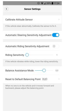
Make sure the "Balance Assistance Mode" is set to 0,0. Failure to do so will result of malfunctioning of the Blumil.
